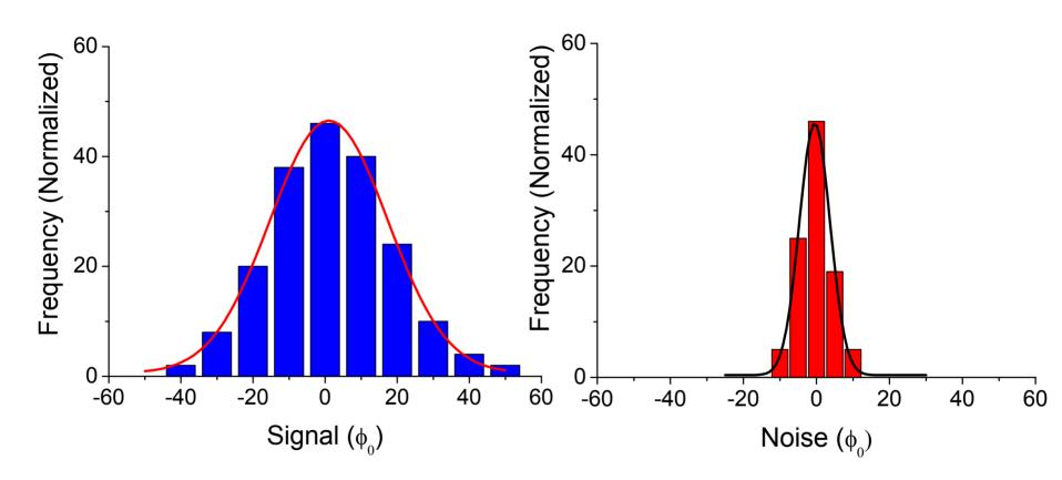
The **signal** histogram is **wider** than the **noise** histogram, and is Gaussian in profile, as expected from the Kibble Zurek scenario.
