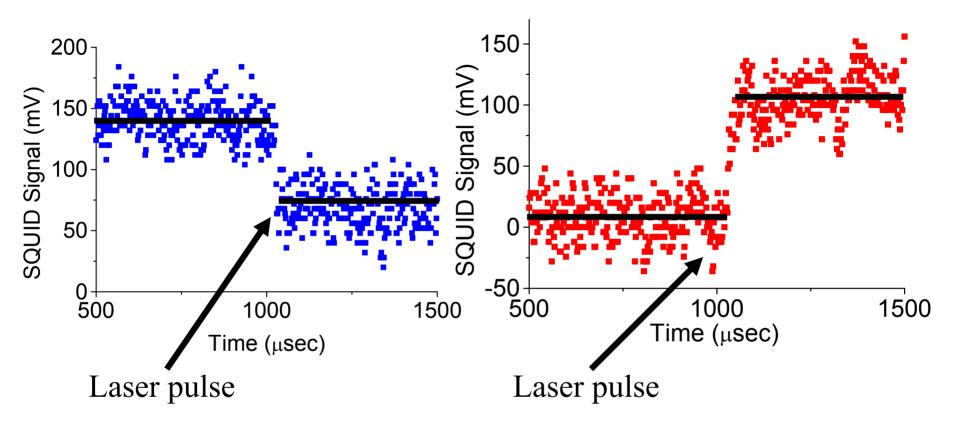
• The dashed lines show the average flux level before and after each measurements.
