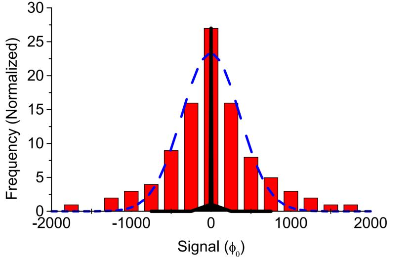
• Gaussian fit to the signal histogram is shown with a blue doted line
