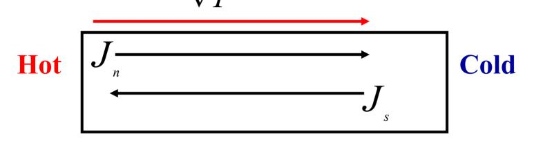
As noted by Ginzburg, in some case such thermo-electric currents can generate magnetic flux. One example is the Anisotropic Thermo-Electric Effect.
