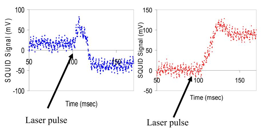
• Contrary to the case of homogenous ilumination, in the hot spot experiments the time scale for the appearance of spontaneous flux is now msec (as compared to  $\mu$  SeC).
