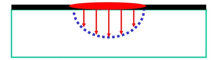
In the second step, the hotter part of the substrate transfers heat to the outer (cold) part of the substrate.
