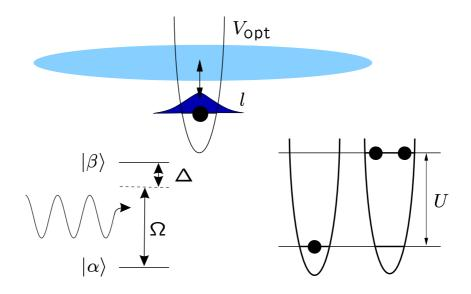
Effective Two-Level System Occupied by Maximally One  $\beta$  Atom
