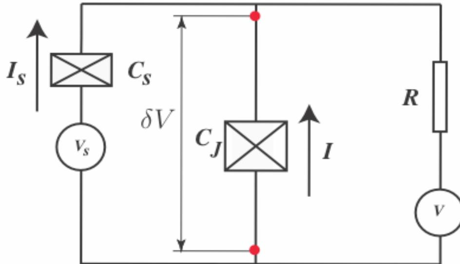
What voltage fluctuation  $\delta V$  is produced by the current fluctuation  $\delta I_s$ ?
